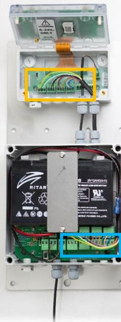
The inputs shown in the blue box connect directly to the inputs in the yellow box on the Metron4 above
